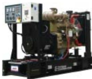
Cummins diesel engine made by DCEC China, Model:6BTAA5.9-G . With radiator at ambient temperature 40°C, fans are driven by belt, with safety guard, With DC 24V charge alternator.
